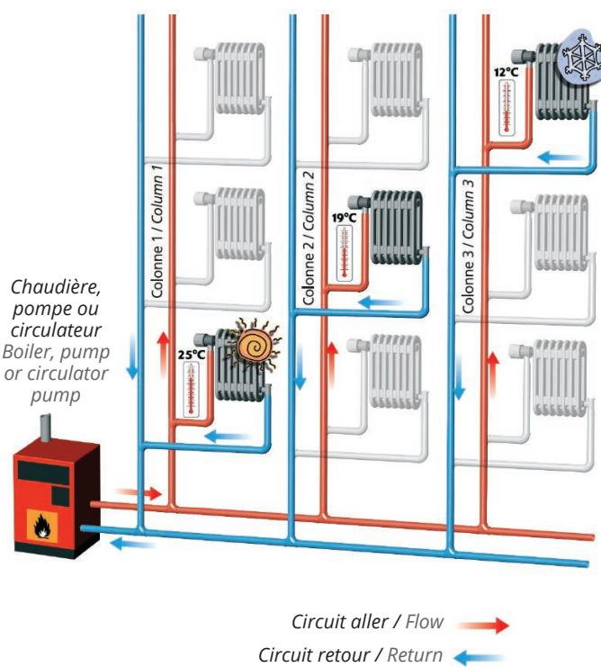
The installation is made up of 3 identical rising columns, without any balancing valves. The flow at exit of boiler is calculated so that each column receives the identical flow.
