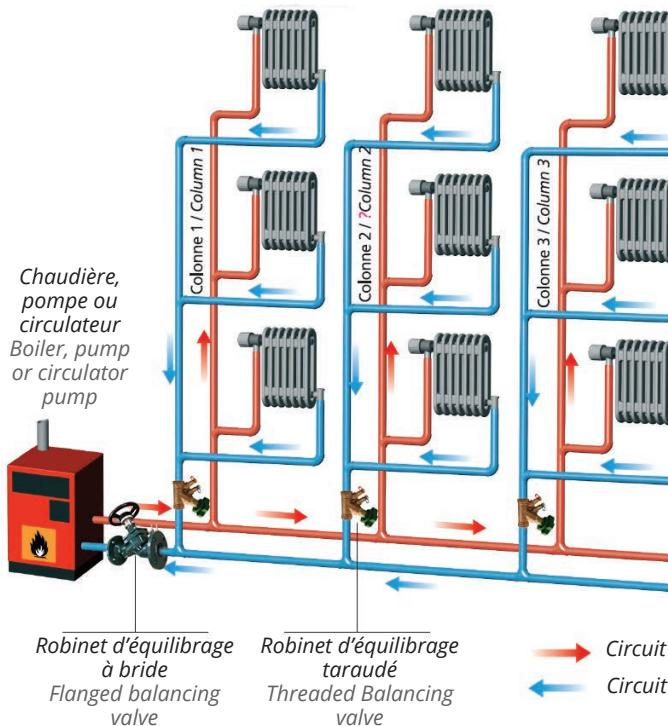
In order to balance the installation, we assemble RC 2106 balancing valves on the return circuits. They will equally distribute the flows in the columns.
